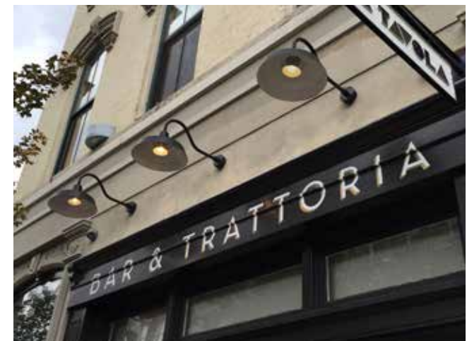
Gooseneck light fixtures can simultaneously provide lighting for signage, the storefront and pedestrians.
