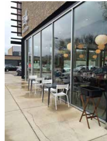
All glass storefronts can be challenging for signage, but this building has a generous solid wall above that allows signage above the entry door, and window signage can be used as a pattern across the storefront.
