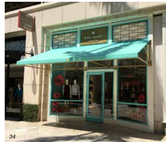
Note the placement and proportion of each element - Awning, Transom, blade sign, building lighting - in order to give each enough room to be visible and functional.
