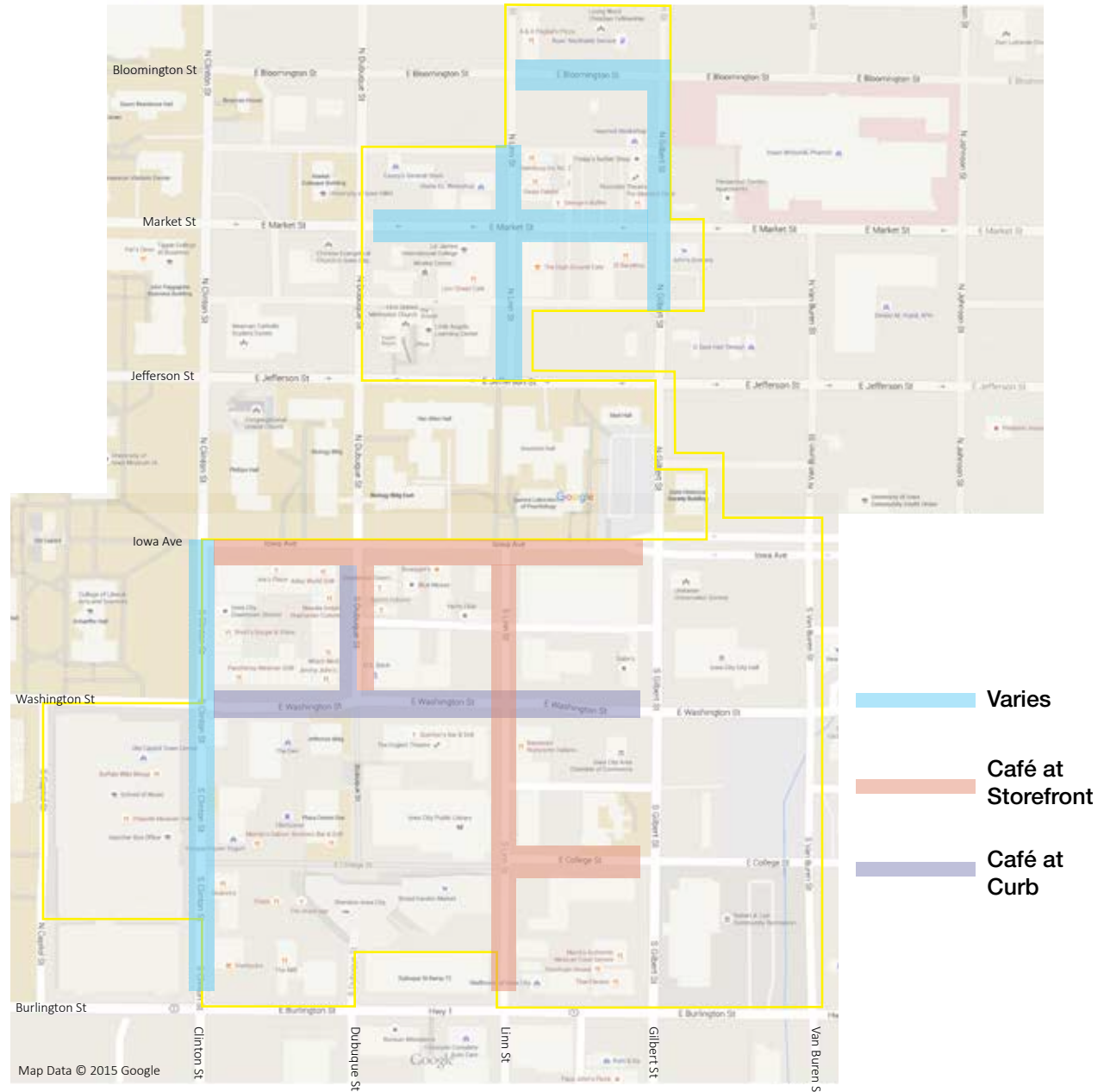
Café Diagram 1: The current desired placement of café seating along streets takes into account the width of the street and sidewalk, and the current placement of cafés. New streetscape configurations may require modifications to the desired placement.
