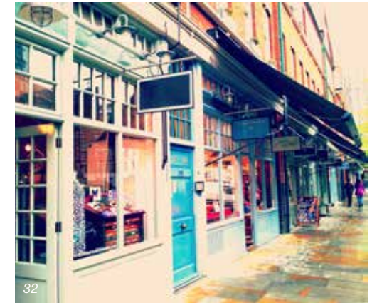
32 Smaller blade signs placed underneath open-ended Awnings are highly visible from the sidewalk.
