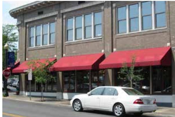
Awnings should respect the architecture; stay within storefront bays and be proportioned appropriately.
